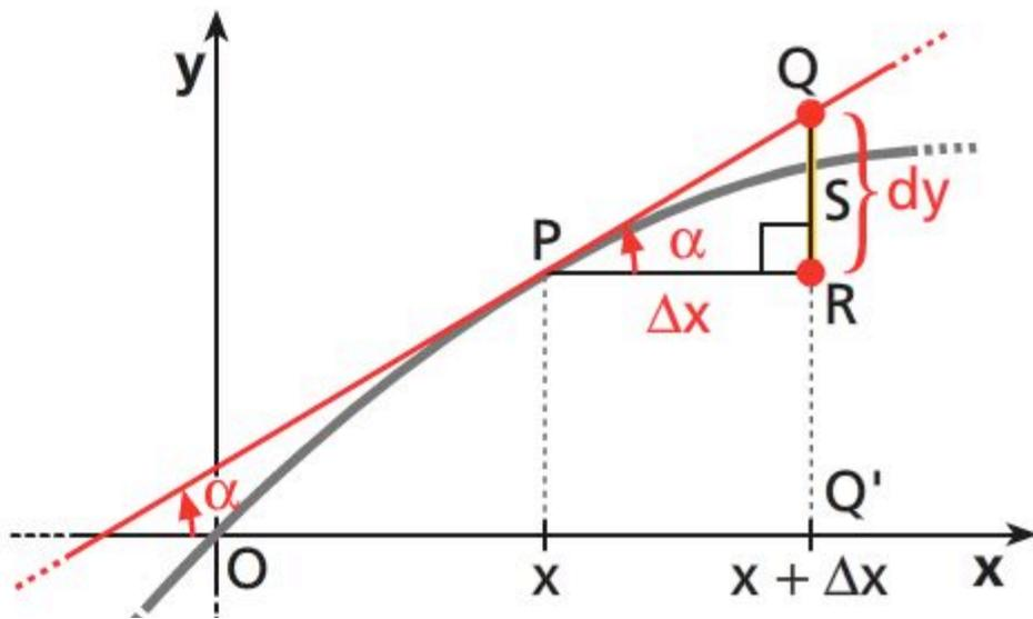
c. Poiché  $\overline{PR} = \Delta x$  e  $\text{tg } \alpha = f'(x)$ , risulta  $\overline{RQ} = dy$ .
